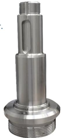
Prior to the install of the Spinner TTC, John Prosock Machine made the part pictured below in seven operations on several different machines in a total cycle time of all combined operations of just over 15 minutes per part.
