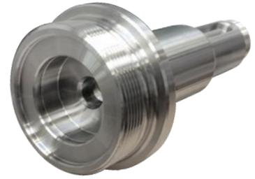
On the Eurotech Spinner TTC they are making the part complete in one operation with a sizable reduction in cycle time. This process includes pinch turning, deep hole drilling, slot milling and threading. The part is machined from bar, which is feed to the machine through the Spinner bar feeder.
