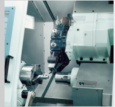
THE TURRET AND WORK ENVELOPE OF THE EUROTECH ELITE 730 SLY MULTI-FLEX
