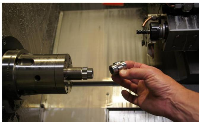
"The cams are the precision part to preset our torque tools. If the cams aren't made perfectly and in one machine operation (which eliminates all these other second ops procedures) then the accuracy of our tool fails. That's another way that we are a leader in the industry. We have the highest accuracy per tool. Some of our competitors are at + or - 6% or -10%. Some of our tools are + or -2%, + or -3%, or + or - 4% which is huge in the industry." - Denise Dobras
